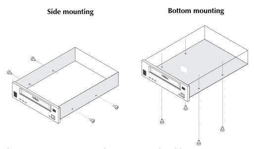
**Figure 2-5** Screw mounting configurations (internal model)
